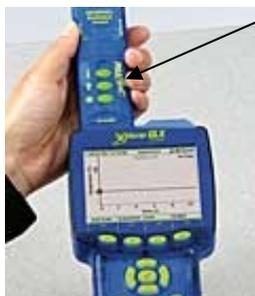
Connect the **sensors** to one of the sensor ports on the top of the GLX.
